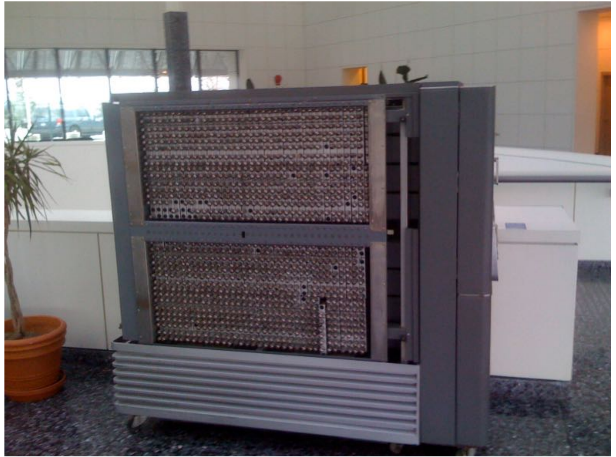
IBM 701 processor frame
