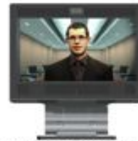
Lifefize Knows includes a 16:9 1280x720 panel display, built-in wide-band conference phone, 8-way audio-video bridge, VGA connection, and a headset jack. The device folds flat for carrying.
